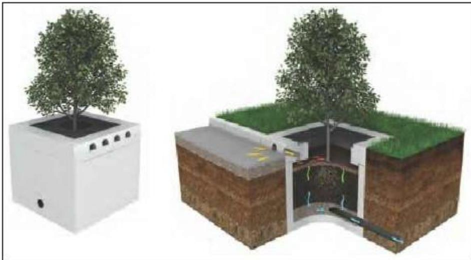
Once surface water makes its way into the tree pit, it will filter down the soil medium. Excess water collected at the bottom of the system will discharge into the existing sewer in the High Street through an outlet pipe. The tree pits will provide a level of surface water treatment via its medium and reduce peak discharges and volumes into Southern Water surface and foul water sewers.
